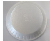
Sample 7—XPS foam disposable plate
