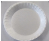
Sample 7—XPS foam disposable plate
