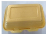
Sample 5—EPS Poly(styrene) takeaway
